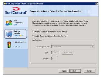
This service is used by SurfControl Mobile Filter to detect when clients are connected to a corporate Web Filter server, which then takes over the filtering of the device from the Mobile Filter client. This service must be installed on the Web Filter server.
